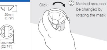
1 Push the mask onto the installed lens
