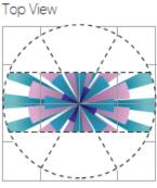
If necessary, the masked area can be altered by cutting off the respective grooved segments with a wire cutter or knife.
